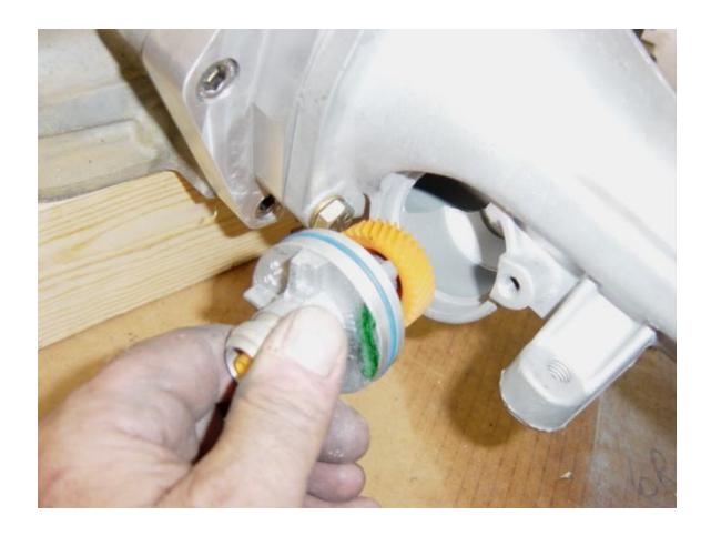
Remove speedometer sleave clamp and install sleave. Install clamp, taking care to position sleave so clamp tangs fit into the sleave properly. Hook-up VSS sensor and mechanical speedometer cable.
