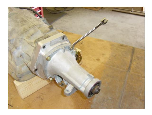
Install tail housing with supplied four bolts.
