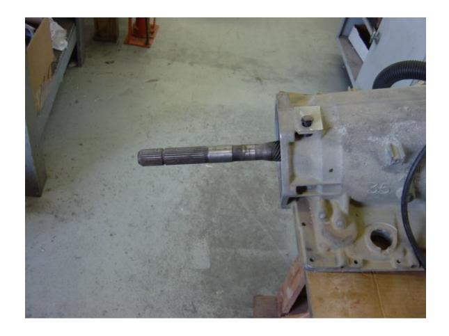
Remove original tail housing and reluctor gear and sleeve. There should be nothing on the output shaft. Retain tail housing o-ring to use on adapter.
