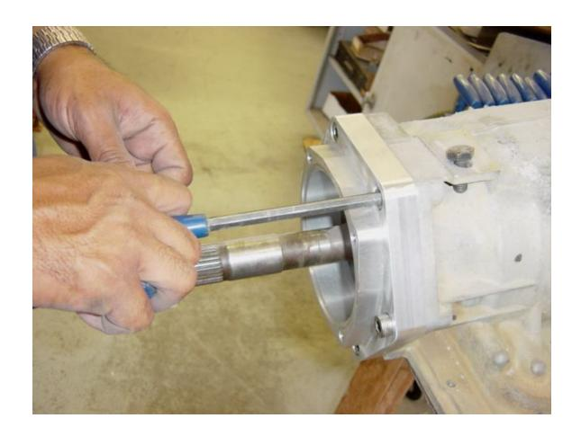
Install original o-ring on 6-bolt adapter. Position adapter on transmission and secure with six stainless cap screws.
