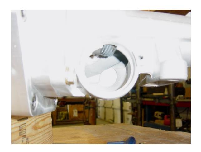
Install tail housing onto adapter with 4 bolts and tighten. Position reluctor/drive gear assembly, so that drive gear is in the center of speedometer sleave opening.
