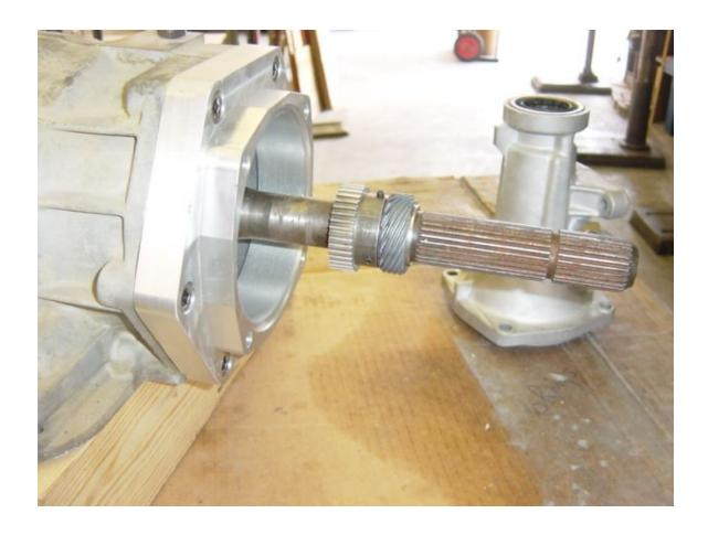
Slide reluctor/drive gear assembly onto output shaft. Do not tighten/set screws. Approximate reluctor/drive gear assembly, so that drive gear is in the center of speedometer sleave opening.
