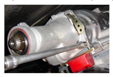
4- Install sleave assembly into extension housing opening. Secure sleave into extension housing with clamp and bolt provided. This completes extension housing installation.
