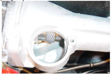
3- Remove extension housing. Being careful not to move the reluctor gear/ drive gear assembly, tighten the three set screws with an allen wrench to secure assembly to output shaft. Install extension housing onto transmission, fasten with bolts, and tighten evenly.
