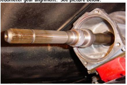
2- Slide tail housing into transmission until seated and visually confirm that the drive gear of the assembly is centered in sleave opening. See picture below.
