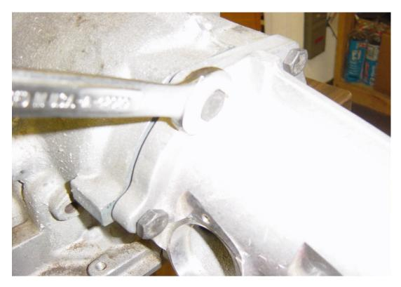
Install sleeve assembly into tail housing. Recommend a small amount of lithium grease on o-ring. Line up retaining clip with tangs on sleeve. Install retaining clip to tail housing using supplied nut.
